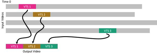
**Figure 4: Illustration of the vehicle tracking query (Q8) on a Visual Road dataset (scale = 1) that contains three vehicle tracking segments (VTSs). Each VTS is temporally-ordered, concatenated, and output.**
